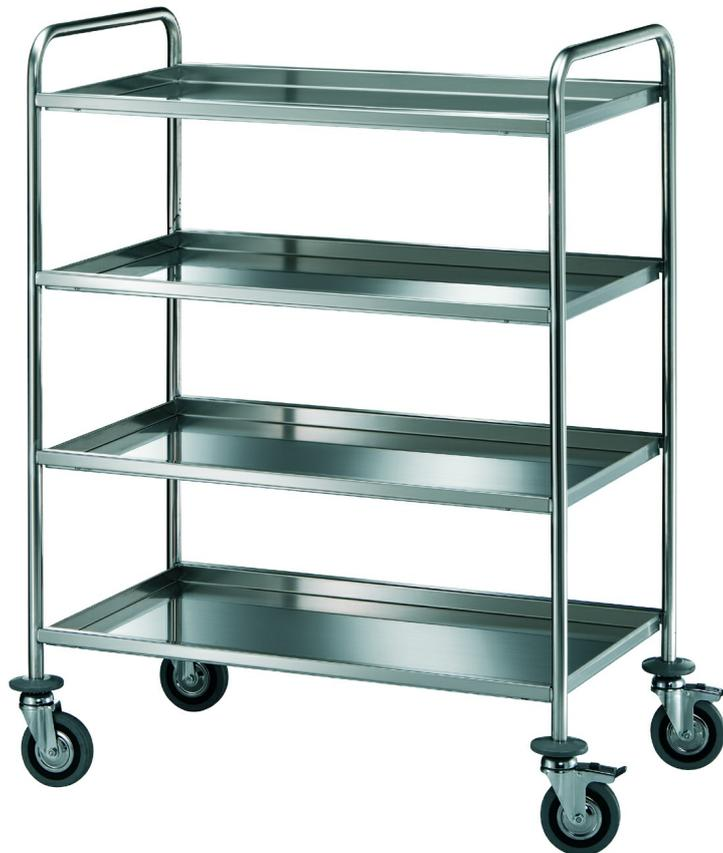
Shelves trolley made in 18/10 stainless steel, welded frame made in stainless steel, round tube  $\varnothing$  25 mm, knit structure, bended shelves h 30 mm. 4 grey rubber swivelling wheels  $\varnothing$  125 mm, rubber bumpers. Four-shelves trolley mm 1020x600x1250h - 419.A
